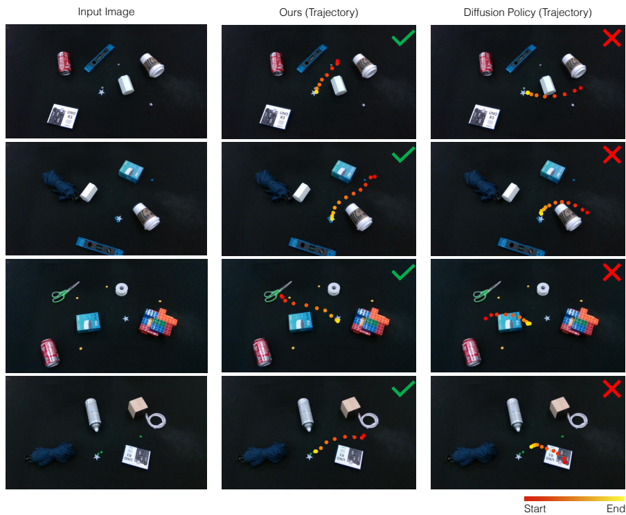
Figure 11: Additional Sweeping Qualitative Results. The trajectory of the end-effector is projected onto the input image.
